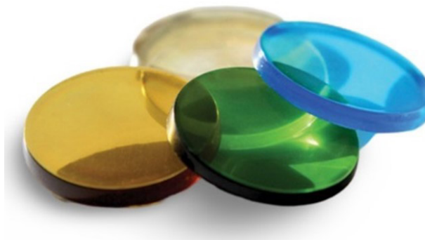
Figure 1. Melted beads with the aid of flux and fusion furnace.
